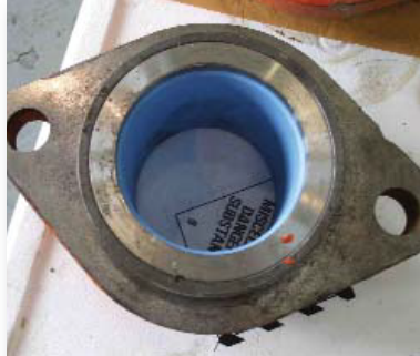
ThorPlas bearing installed in retaining lip
