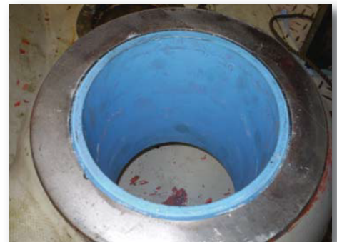
White Rock refits with grease free ThorPlas bearings
